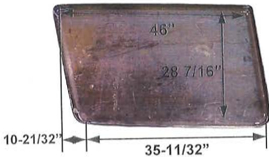
DA Part # : DA- 76035 Ref # : AVAILABLE IN VARIOUS SIZES Description: HOPPER DOOR, TRAP. RH
